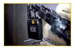
Light weight relay with MESH network communication
